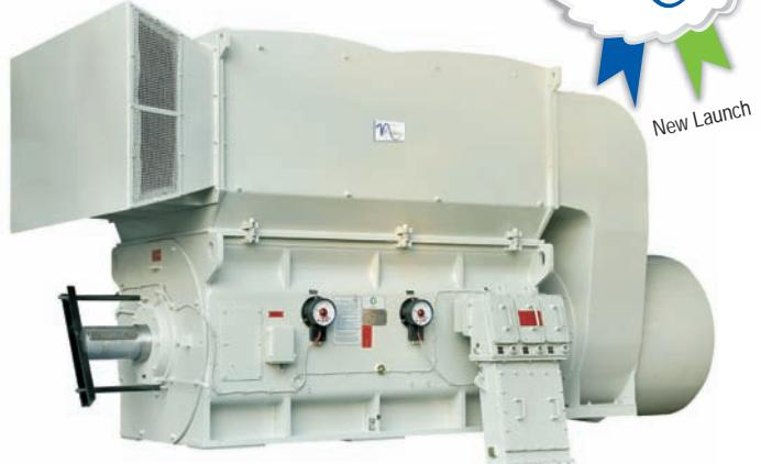
2550kW, 6Pole, 11KV, 560 Frame, Fan Drive, Induction Motor
