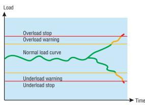
CG M20 shaft power monitor protects your equipment and process against damage and downtime. Early warnings and stops allow preventive action.
